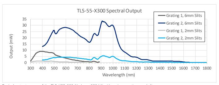
Typical output power of the TLS-X55-300 (Xe lamp 300 W) with various gratings and slits
